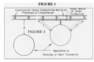
"B" equals the reduced clearance permitted in accordance with Table 2. The protection, applied to the construction using combustible material, should extend far enough in each direction to make "C" equal to "A".
